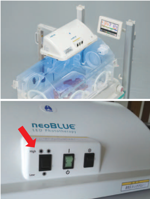
Figure 2 neoBLUE® The switch the arrow is pointing at changes between the High and Low modes.
